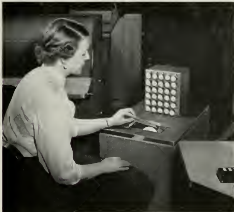
Largest installation yet of "TV Eye" helps to speed banking operations at the Provident Institution for Savings in Boston. File clerk, above, holds signature card before the camera for viewing by teller, right.
