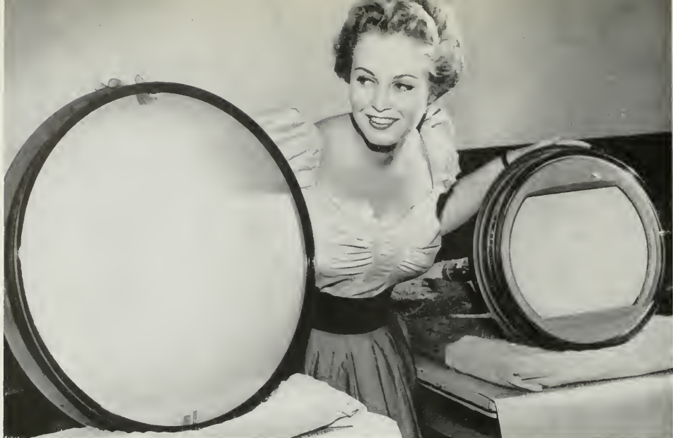
RCA's new 21-inch color TV tube is shown here in comparison with the earlier 15-inch color tube introduced by RCA in its first commercially-produced color television sets.
